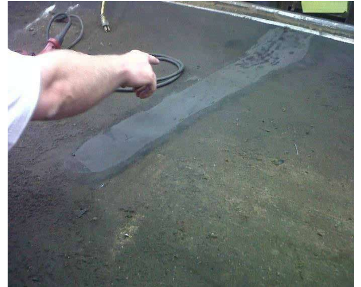
Rapid cure time allowing for normal use of conveyor belt in as little as one hour.
